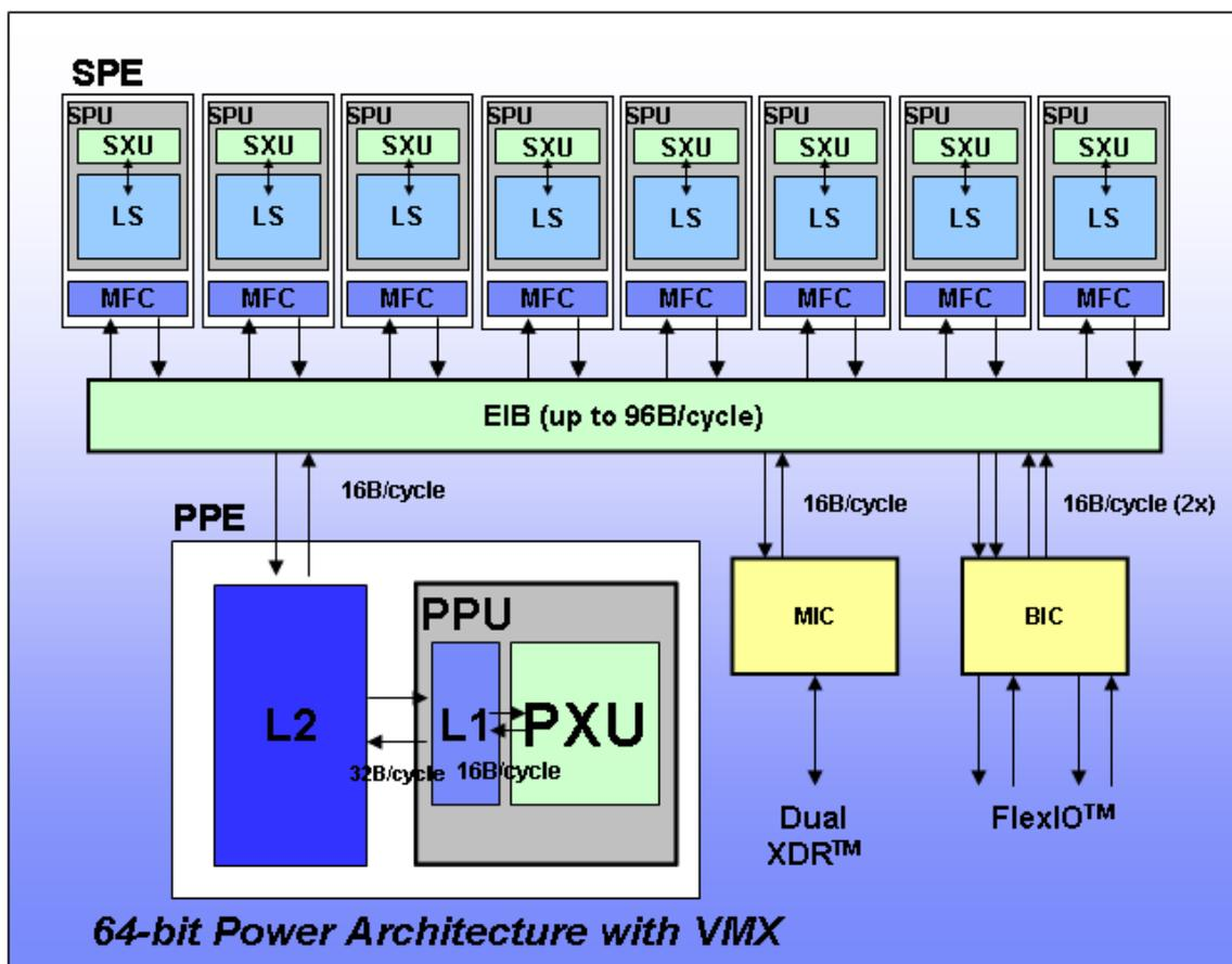
Fig. 6 – The intern architecture of CELL processor used in central system MASMED
