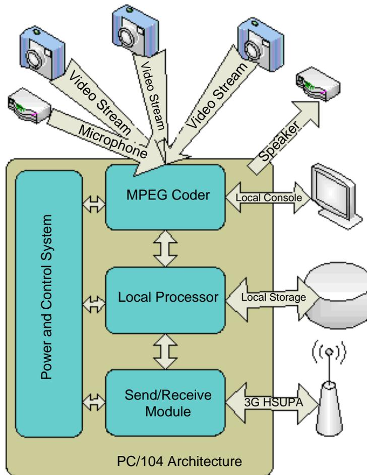
Fig. 2 - The structure of the system for control and command of the equipment of the mobile platform (ambulance)
